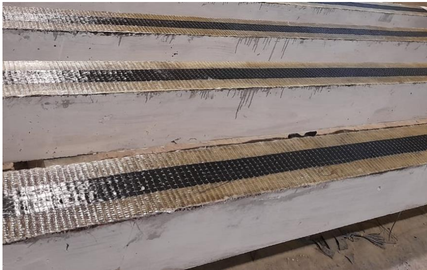
Figure 4. Hybrid FRP strengthened beam
